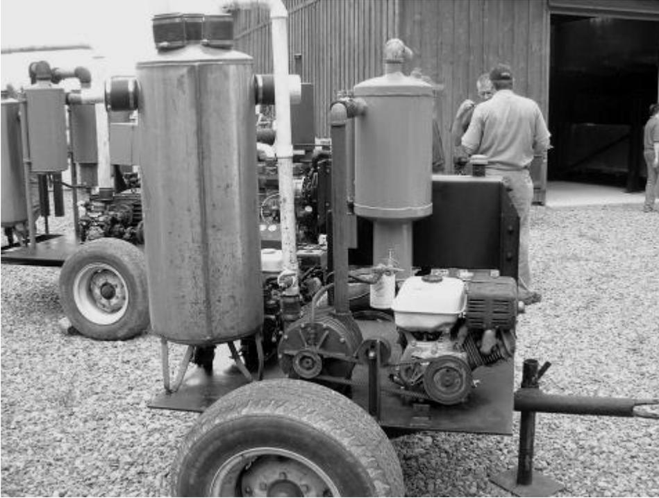
Gas powered vacuum pump on a trailer
