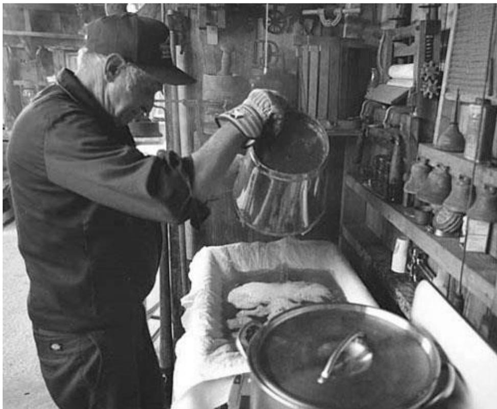
The flat filters allow for greater filtering surface area. The paper and the felt should each lay on their own grill or screen. They function better if the paper is not laying directly on the felt.
